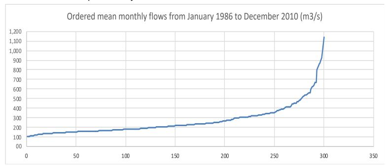
In the Figure it can also be seen that even the 130 m3/s average monthly flow was exceeded almost every month since the starting of the operation in Dniestrovski HPP 2 and reservoir, which was not the case before. Once again, a probability of exceedance should be considered, 84% being proposed.
